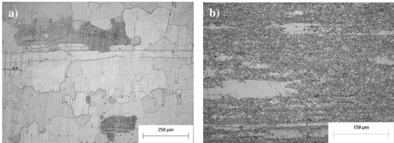
Figure 1. Microstructure of the as-extruded alloys; a) alloy 0; b) alloy 2.
