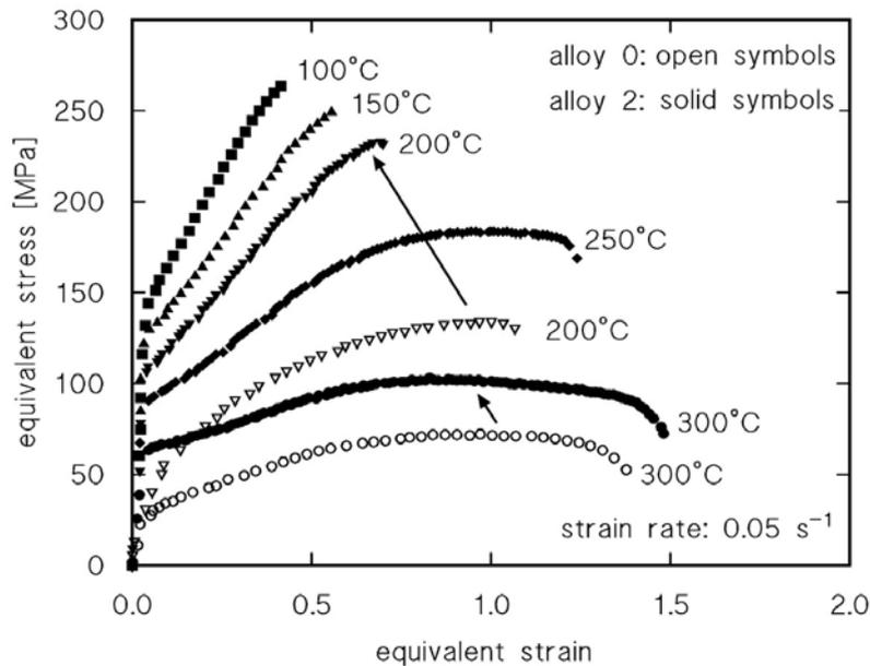
Figure 2. Comparison between the equivalent stress vs equivalent strain obtained by testing the two alloys under a strain rate of  $0.05 \text{ s}^{-1}$ .
