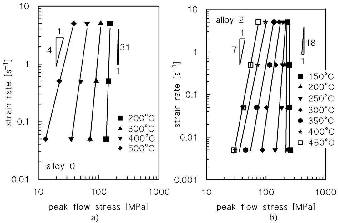
Figure 3. Peak flow equivalent stress as a function of the testing strain rate (torsion testing) for the two investigated alloys.
