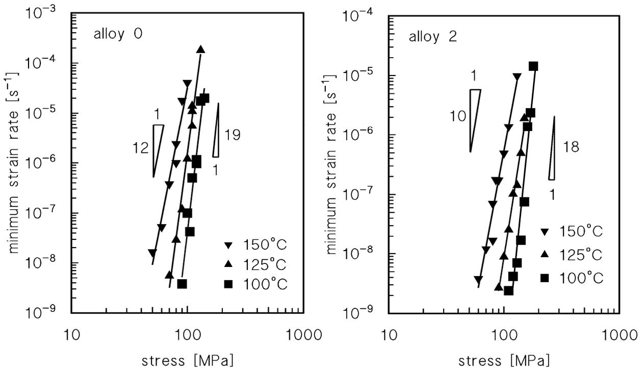
Figure 4. Minimum creep rate as a function of applied stress for the two alloys.
