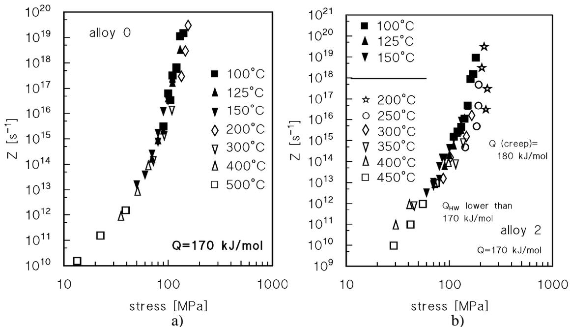
Figure 5. Zener-Hollomon parameter as a function of stress for both tensile creep and torsion data. The same value of the activation energy ( $Q=170$  kJ/mol) was used.
