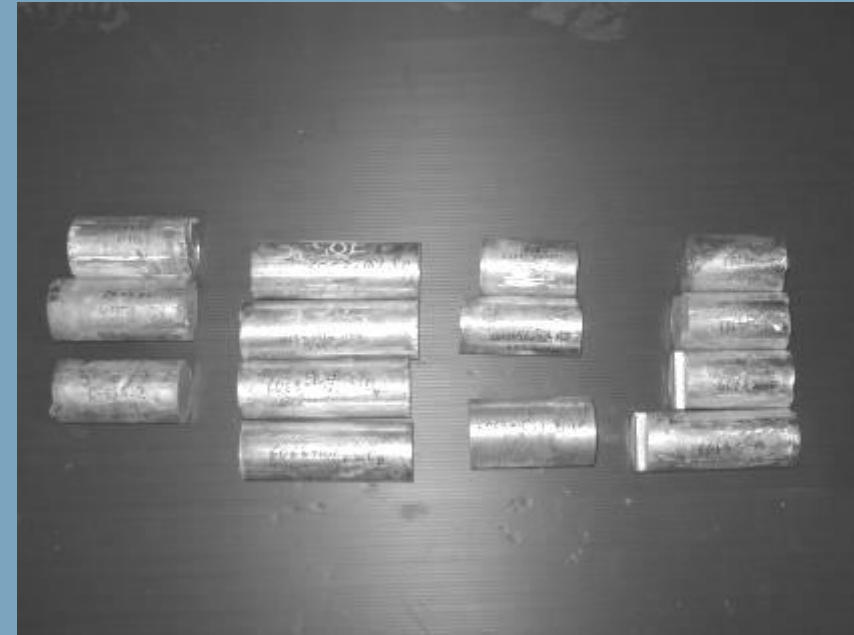
Cast AZ31 cylinders reinforced with 5%-30% SiC particles as raw material for extrusion.
