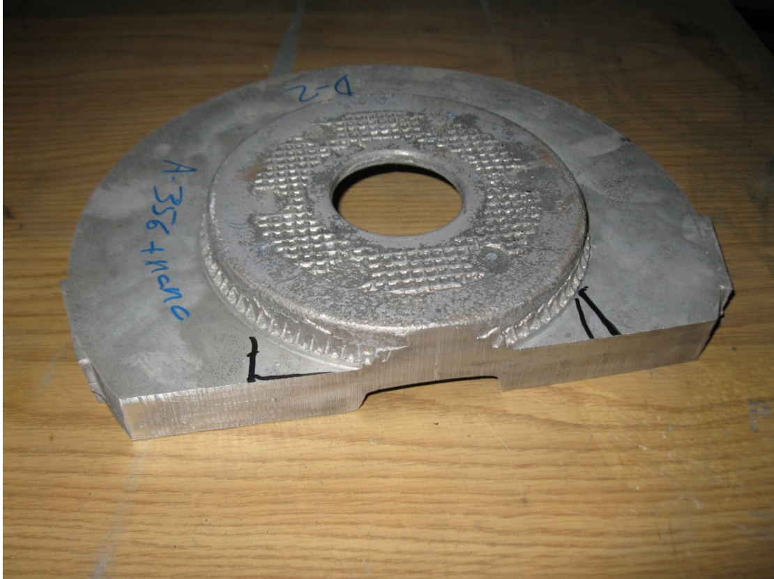
Fig.1 . The disk after cutting out tensile specimens.
